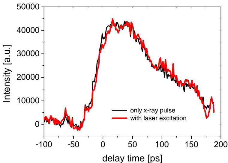
Fig 2: Traces of the scattering from 60nm gold particles supported on a silicon wafer as function of time. There is a slight change in scattering after the laser impact on the particles (delay time 0), which may reflect the lattice disturbance.
