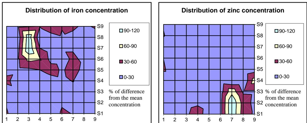
**Figure 1:** Variation of Fe and Zn concentrations within a specimen
