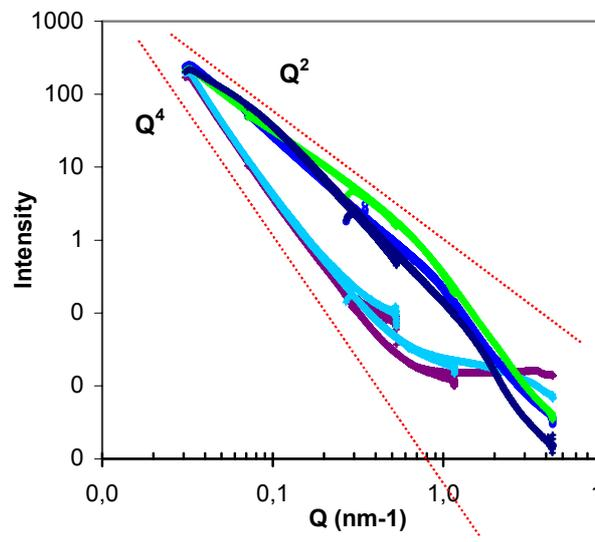
Fig. 2. SAXS plots of nanocomposites containing (1) needle like particles, (2) rod like particles, and (3) spherical particles.
