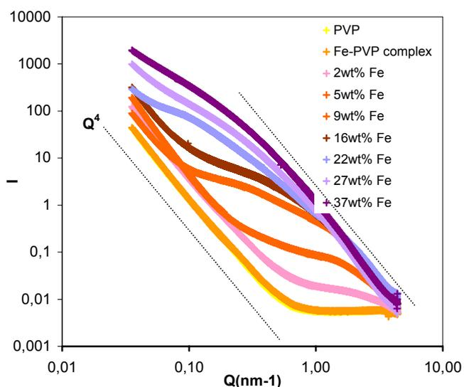
Figure 3. Scattering plots of nanocomposite samples prepared from different iron/polymer ratios.
