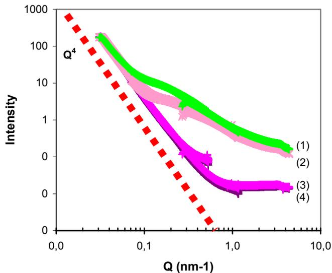
Fig. 1. SAXS plots of (1) as prepared nanocomposite film, (2) PVP polymer pellet, and (3) Fe-PVP coordination compound.
