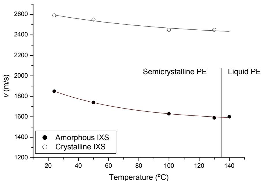
**Figure 2.** Sound velocities inferred from dispersion curves of the inelastic X ray scattering contributions of amorphous and crystalline phases of polyethylene at different temperatures, below and above complete melting of the crystallites. Lines are guides to the eye.
