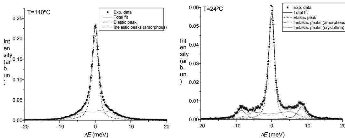
**Figure 1.** Inelastic X ray scattering spectra of liquid (left) and semicrystalline (right) polyethylene.
