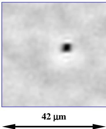
Fig. 3: Phase images showing probably an “inclusion”. Pixel size  $0.33\ \mu\text{m}$ , beam energy  $24\text{keV}$ , reconstructed from 4 images at distances 12, 20, 45, 100mm
