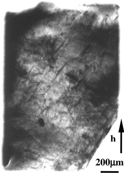
Fig. 1: Reflection  $\tau^3(0/2\ 0/0\ 0/0)$ , 2-fold axis, rocking angle  $0.025^\circ$ , sample-to-film distance  $d_{s-f} = 4\text{cm}$ , beam energy  $24\text{keV}$ . **h** - diffraction vector. Contrasts due to global bending, dislocations, pores and two-dimensional defects visible.
