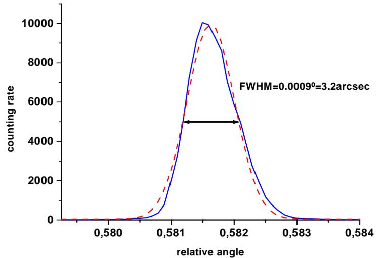
Fig. 2: Measured rocking curve (straight line) in a  $50 \times 50\ \mu\text{m}^2$  field, reflection  $(0/2\ 0/0\ 0/0)$ , together with a Gaussian fit (dotted line), full width at half maximum (FWHM) is about  $0.0009$ degrees
