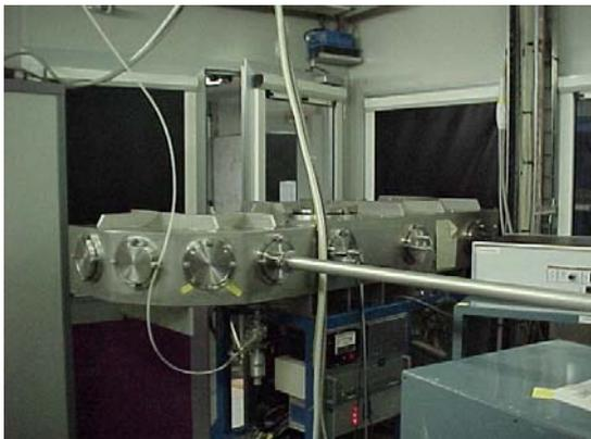
Fig. 1: Photograph of the von Hamos spectrometer as installed at the ESRF beam line ID21.
