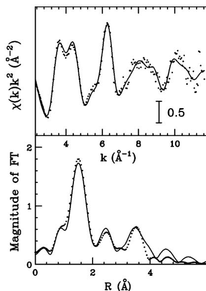
FIGURE 6: EXAFS fitting results of the Cu(II)/His-rich complex. Upper panel: Comparison of the theoretical signal (solid line) with experimental data (dotted line) of Cu K-edge  $k^2$ -weighted EXAFS data of Cu(II)/His-rich aqueous solution. Lower panel: Nonphase-shift-corrected Fourier transforms of the experimental data (dotted line) and of the total theoretical signal (solid line).
