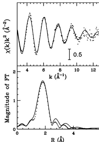
FIGURE 4: EXAFS fitting results of the Cu(I)/Met-rich complex. Upper panel: Comparison of the theoretical signal (solid line) with experimental data (dotted line) of Cu K-edge  $k^2$ -weighted EXAFS data of Cu(I)/Met-rich aqueous solution. Lower panel: Nonphase-shift-corrected Fourier transforms of the experimental data (dotted line) and of the total theoretical signal (solid line).
