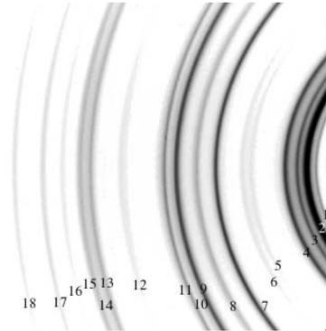
*2d spectrum of samples from series A with 32 % of deformation where the three phases are present*
