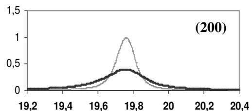
*Spectrum (point detector) of slightly deformed (gray) and highly deformed (bold) of samples of series D and E. We can notice a shift of the (111)  $\gamma$  peak (left) whereas the (200)  $\gamma$  peak(right) remains at the same position*
