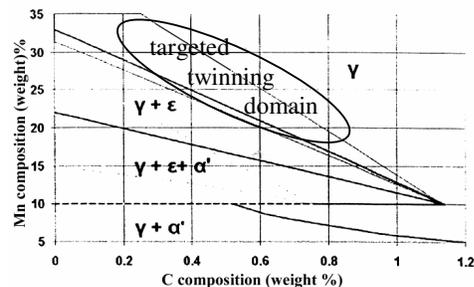
Figure 1 : Structural state of the steel after deformation at room temperature, as a function of Mn and C composition.
