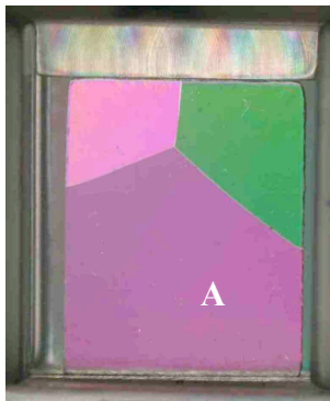
Figure 1 : Photograph of a tri-crystal, with cross-polarized light. (A : studied grain shown on figures 2 and 3)
