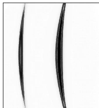
Figure 1: CCD image of transmitted Debye-Scherrer rings of (111) and (200) peaks of the 10% deformed alloy 1.
