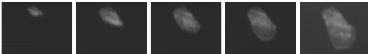
Fig. 6. Projection of a diffraction spot in a near field detector of a growing recrystallization nucleus into a 30% cold rolled Cube matrix growing at 300°C, snapshots at time = 0 s, 585 s, 990 s, 1530 s and 2200 s. The width of each image is 500 \mu\text{m} .
