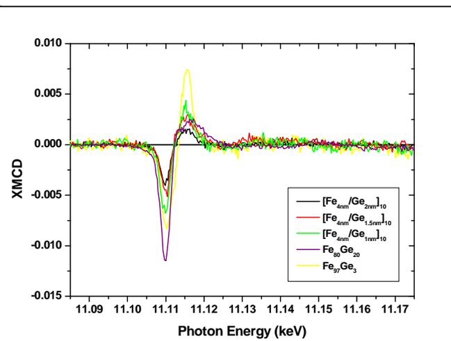
**Fig.2:** Ge K-edge XMCD spectra for various  $Fe_n/Ge_m$  magnetic multilayers and  $Fe_{1-x}Ge_x$  alloys. The spectra have been recorded at 10K and under 2Tesla external magnetic field.
