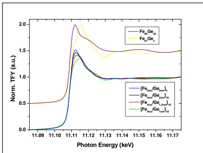
**Fig.1:** Isotropic normalized Ge K-edge XANES spectra for various  $Fe_n/Ge_m$  magnetic multilayers and  $Fe_{1-x}Ge_x$  alloys. The XANES spectra for the alloys have been shifted by 0.5 for clarity of presentation.
