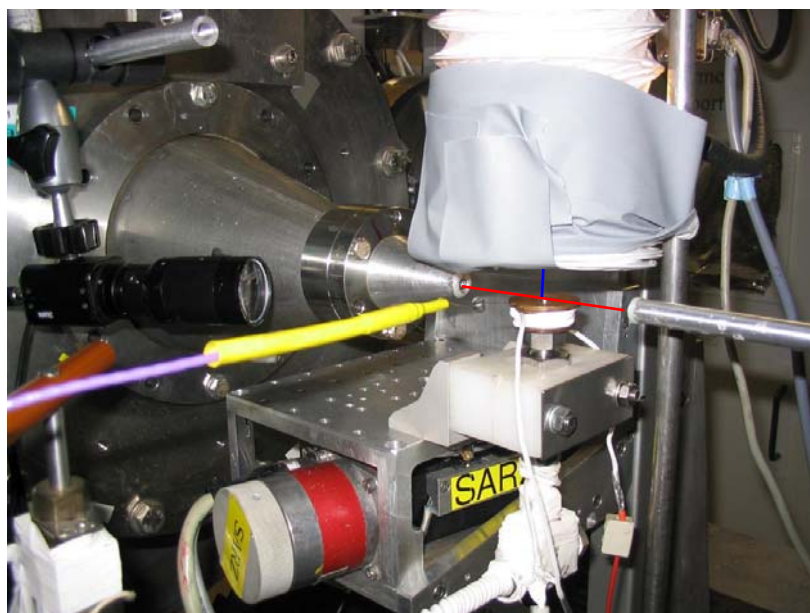
Figure 2 The heated nozzle mounted on the positionig table in front of the SAXS pinhole camera setup. The red line indicates the position of the x-ray beam, the blue line the position of the jet from a 50 \mu\text{m} nozzle.
