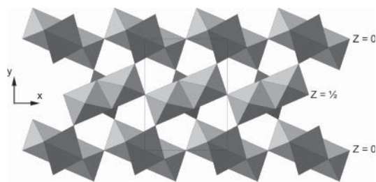
Figure 7. Projection of the crystal structure of \gamma\text{-AlH}_3 along [001] shown as a packing of the \text{AlH}_6 octahedra. Large cavities in the structure are clearly seen.
