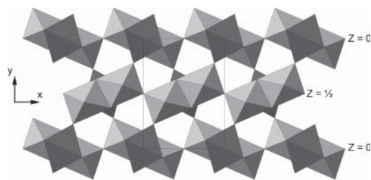
Figure 7. Projection of the crystal structure of \gamma\text{-AlH}_3 along [001] shown as a packing of the \text{AlH}_6 octahedra. Large cavities in the structure are clearly seen.
