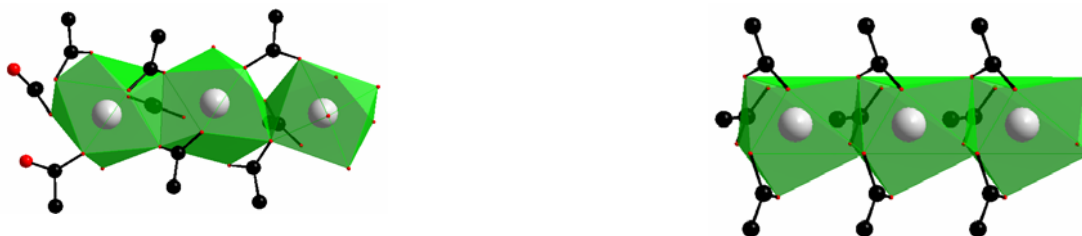
Change in the Eu coordination in MIL103-Eu: before (left) and after (right) outgassing.
