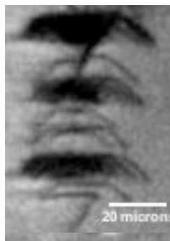
(a) after first T - C cycle (b) T , 30 mn : 5 MPa @ 680°C (c) C, 3 mn : 5 MPa @ 680°C
