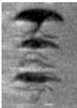
(a) after first T - C cycle (b) T , 30 mn : 5 MPa @ 680°C (c) C, 3 mn : 5 MPa @ 680°C
