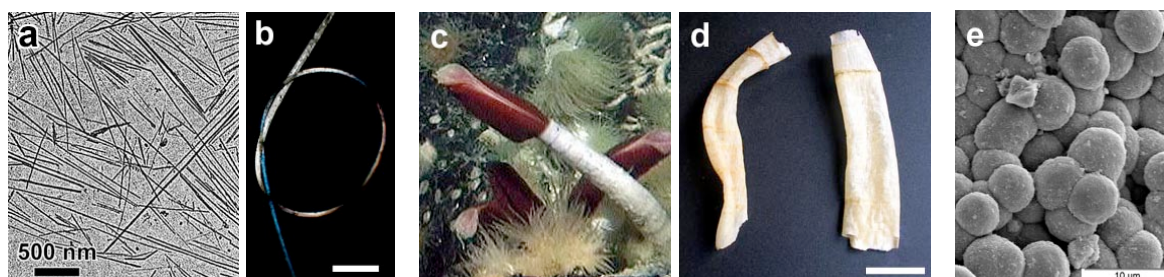
Figure 1. a ) Tunicate cellulose whiskers (TEM image - bar : 100 nm) ; b ) artificial fibers containing aligned cellulose whiskers (bar : 5 mm) ; c ) Tevnia vent worm photographed close to a deep sea hydrothermal source ; d ) dry tubes from Tevnia worms containing highly crystalline chitin microfibrils (bar: 2 cm) ; e ) highly crystalline starch spherocrystals (SEM image).
