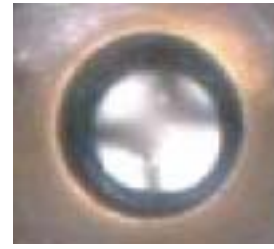
Fig.2. Conoscopic image of the homeotropic N phase of ODBP-Ph-OC 4 .
