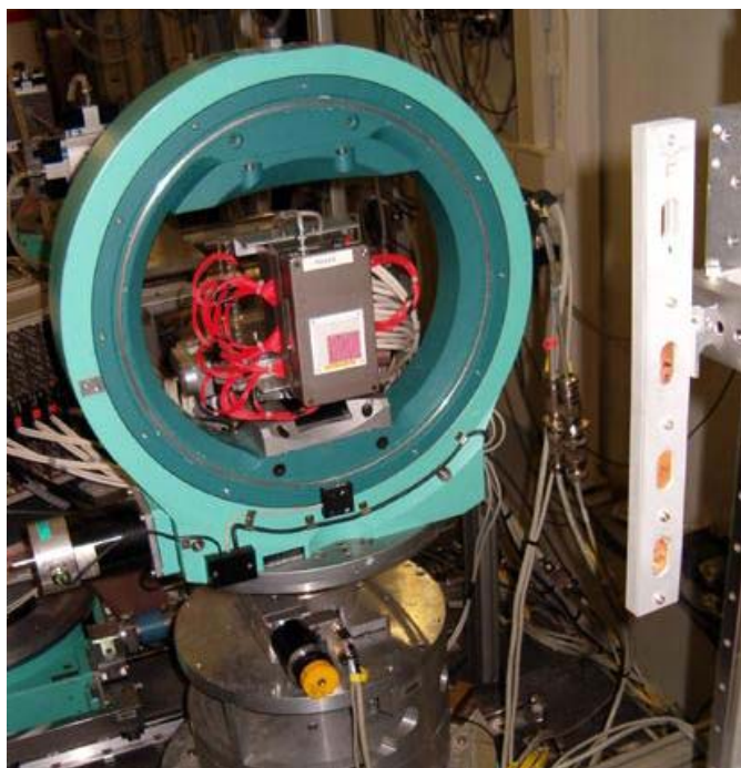
Figure 10. The ID 15A setup for test with Cu crystals in Laue diffraction configuration and the POLCA II detector. On the right the Cu crystals holder. Crystal planes are parallel to the long side of the holders (280 mm). The Al holder accommodates 3 crystals with thickness varying from 6 to 7.3 mm.
