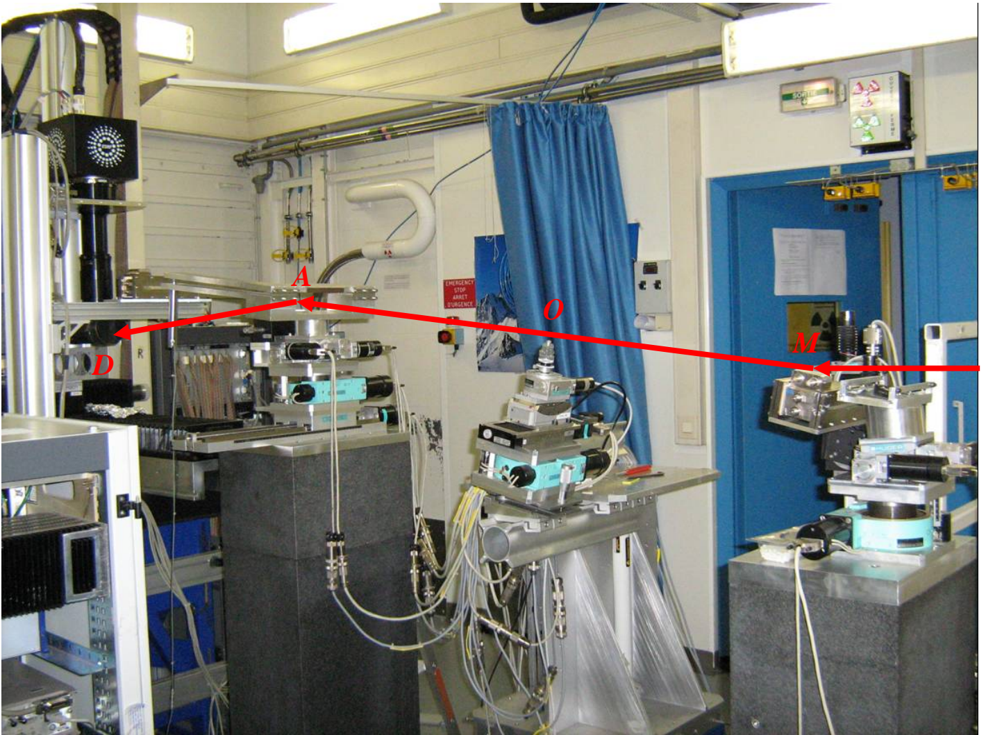
Fig.2 Photograph of the experimental setup. M – single-crystal monochromator, O – object stage with optional vertical (horizontal) rotation axis, A – single-crystal analyser, D – detector.
