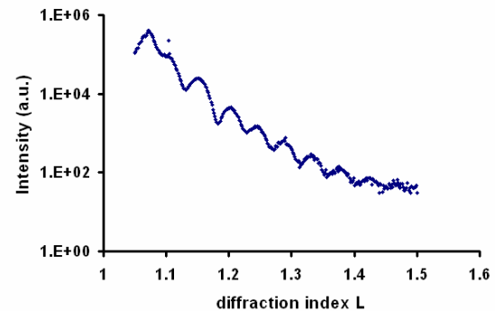
Fig 3 Kiessig fringes around the 001 reflection. The distance of the fringes is related being to the number of monolayers.
