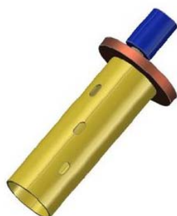
Figure 7: CAD drawing of an improved cryo-SAXS sample holder. The thermal shielding is facilitated by a metal cylinder with beam entrance and exit windows. The cylinder is moveable by a cryogenic adapted motor.
