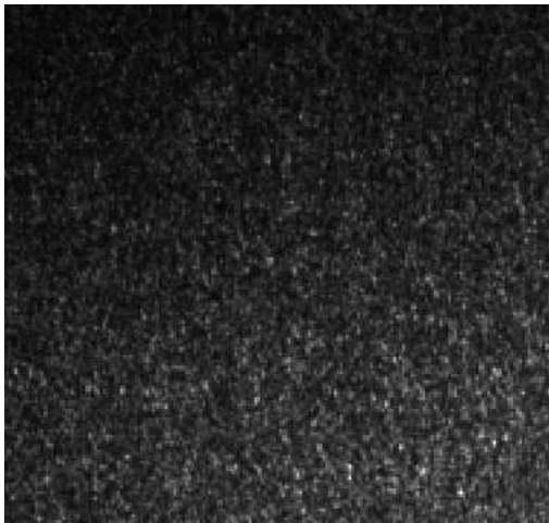
Figure 1: SAXS of Ag precipitates in glass. Detail of 1000 summed frames, from q = 0.044\text{ nm}^{-1} (right bottom) to q = 0.166\text{ nm}^{-1} (left top).
