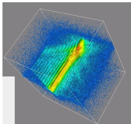
Fig.4: 3D Bragg peak of the same grain (31 2D slices in omega)
