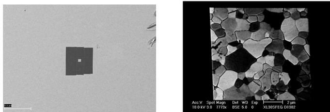
*Fig.1: Special design of the sample allow us to know which grain is mapped*
