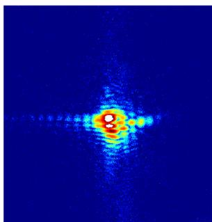
Fig.3: 2D slice of (111) Bragg Peak of an <111> oriented grain at T=50°C
