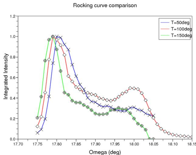
Fig.2: Rocking Curve Evolution in Temperature
