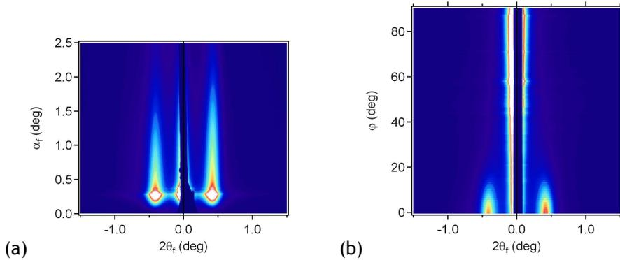
Fig. 1: (a) Out-of-plane (at  $\varphi = 0^\circ$ ) and (b) in-plane (at  $\alpha_f = 0.4^\circ$ ) GISAXS maps of an as-etched  $\text{Si}_3\text{N}_4$  film.
