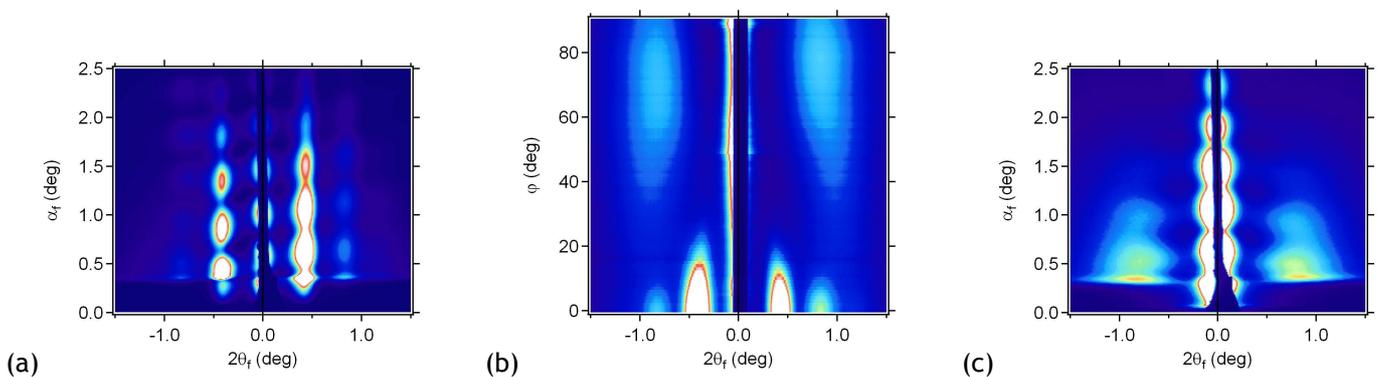
Fig. 2: (a) out-of-plane (at  $\varphi = 0^\circ$ ) and (b) in-plane (at  $\alpha_f = 0.4^\circ$ ) GISAXS maps of  $\text{Al}_2\text{O}_3$ -capped Ag nanoparticles deposited onto an etched  $\text{Al}_2\text{O}_3$  film. (c) Out-of-plane GISAXS map with  $\varphi = 90^\circ$ .
