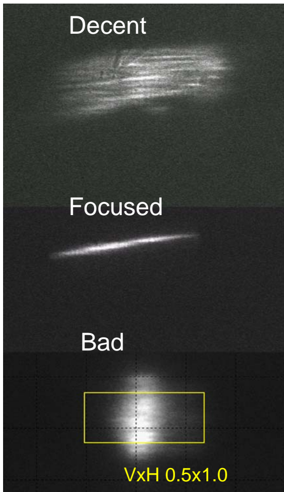
Figure 8. X-ray white beam topograph (in transmission) of a beamsplitter diamond plate installed at ID10B (above) and three pictures of the beam several meters after the crystal
