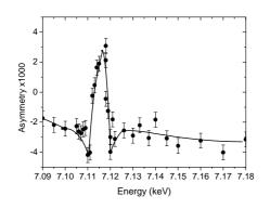
The amplitude of the magnetic effect is about 0.007 as expected by a non dipolar electronic transition (1s-3d). The base line of the curve is centered at approx. -3 E-3 instead at 0. The origin of this phenomenon is not understood at the moment.
