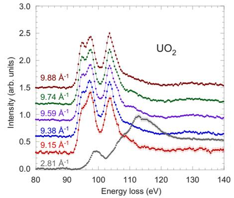
FIG. 2. (Color online) NIXS spectra measured for  $\text{UO}_2$  at the uranium  $O_{4,5}$  edges with a fixed final energy of 9.689 keV, at different values of the scattering vector  $q$  as indicated. The NIXS signal has been normalized to the peak centered at 104 eV in the high- $q$  spectra.
