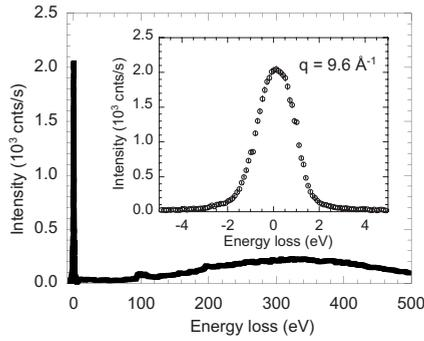
FIG. 1. Photon energy-loss spectrum measured for  $\text{UO}_2$  at room temperature over an extended energy range including the elastic and Compton peaks. Data have been collected with a fixed final energy of 9.689 keV, at a transferred wave vector  $q=9.6 \text{ \AA}^{-1}$ . The inset shows the elastic peak, whose full width at half maximum is 1.3 eV.
