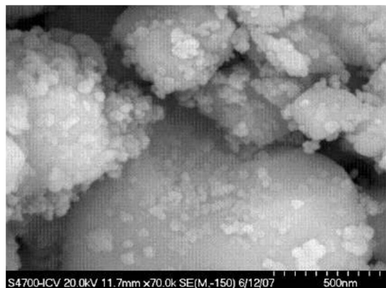
FIG. 2. FE-SEM micrograph for the 5% \text{Co}_3\text{O}_4 –95% ZnO sample after milling showing the \text{Co}_3\text{O}_4 particles dispersed over the surface of large ZnO ones.
