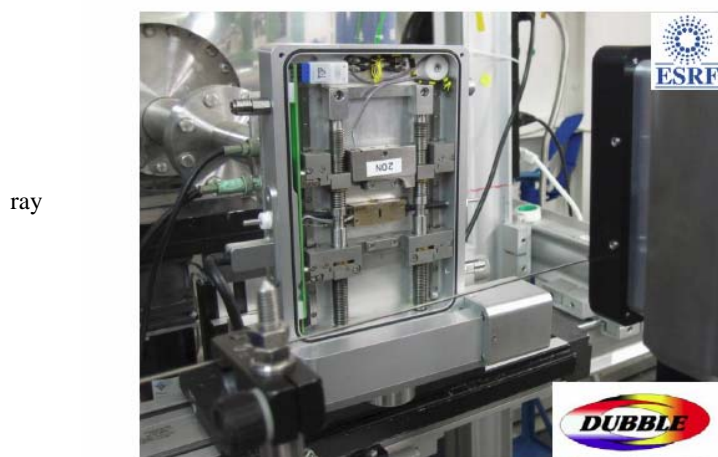
Figure 1: Top, Linkam instrument mounted in the X-beam; bottom, example of specimen positioned in the Linkam tensile device
