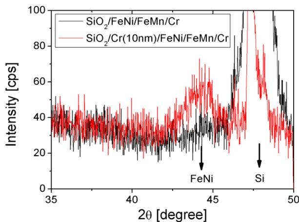
Fig. 1. GID pattern of magnetic multilayered structures representing the better crystalline quality of permalloy film grown on 10 nm Cr buffer layer.
