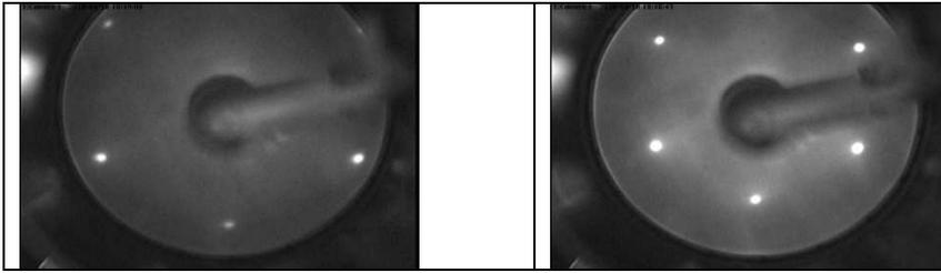
**Figure 1:** Sharp LEED patterns of the single crystalline Ag(111) surface as prepared during the experiment for primary electron energies of 69eV (left) and 140eV (right).
