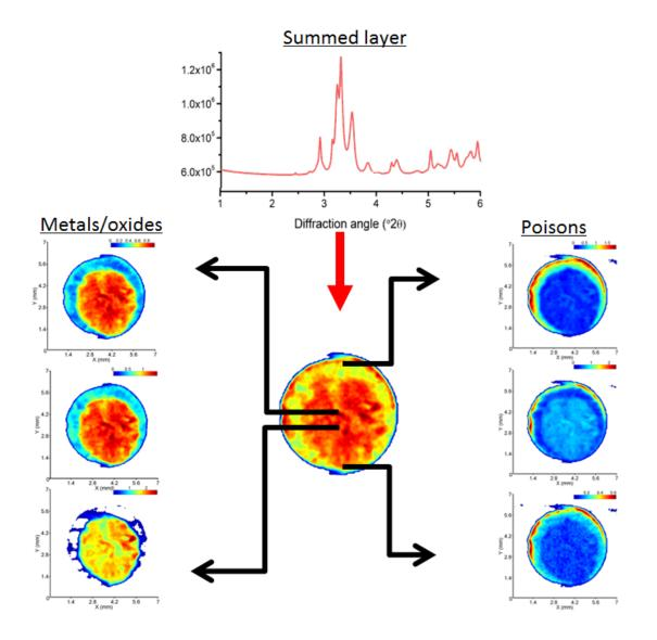
**Figure 1:** Demonstration of some of the data obtained from this beam time. The image shows how the spatial details form the summed diffraction image of the entire layer can be obtained using back projection algorithms, allowing us to observed the distribution of various metals, oxides and poisons within an cylindrical industrial catalyst body.
