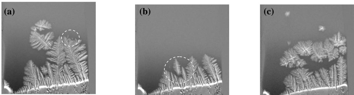
Figure 2: a) Secondary arm fragmentation. b) Primary trunk detachment. a) and b) Al-14wt%Sn solidified with a cooling rate of 8K/min. c) CET in Al-14wt%Sn solidified with a cooling rate of 16K/min.(width of the images= 6mm)
