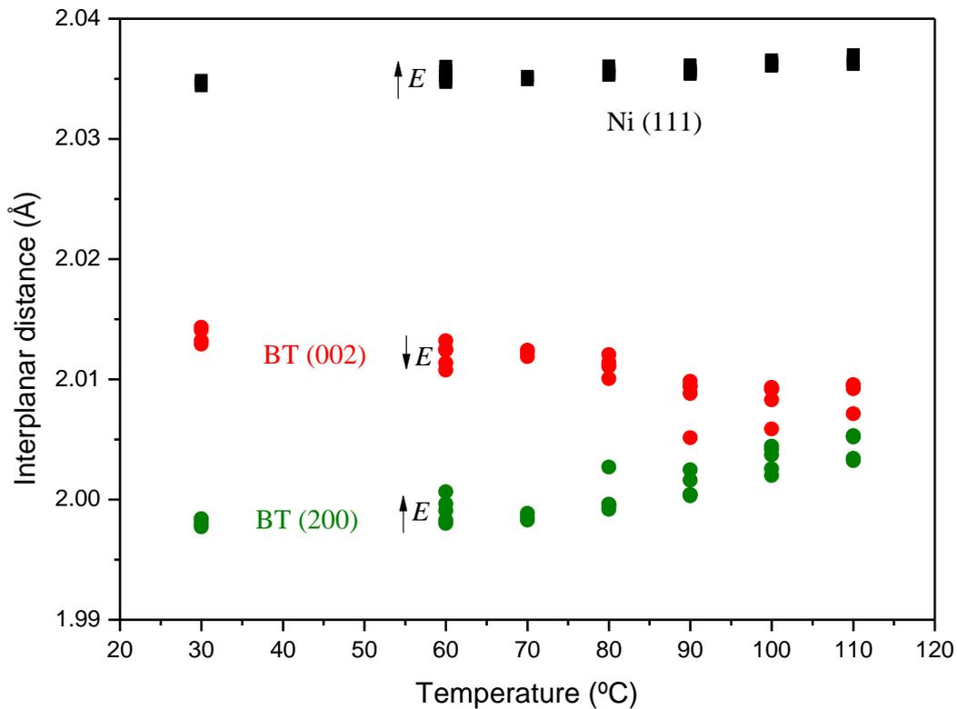
Figure 1: Variation of (002) and (200) interplanar distance in BT ( red and green circles, respectively) and (111) in Ni( black squares ) vs. temperature under different external electric field for a 28% Ni/BT sample. Arrows indicate the increasing external electric field.
