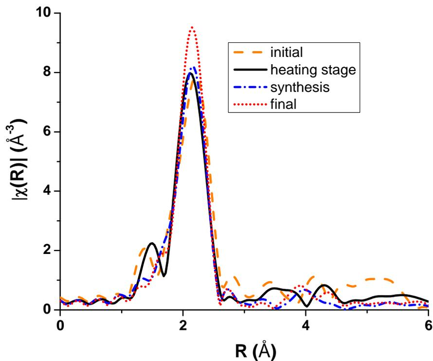
Figure 3.4:  $\chi(R)$  plot of ZnS synthesis experiment analogous to curved wires synthesis conditions: the initial powder mixture is marked in dashed orange, the heating stage is marked in solid black, the synthesis stage is marked in dot-dashed blue and the final state is marked in dotted red.
