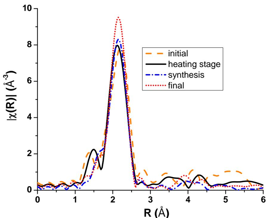
Figure 3.5:  $\chi(R)$  plot of CdS synthesis experiment analogous to tripods synthesis conditions: the initial powder mixture is marked in dashed orange, the heating stage is marked in solid black, the synthesis stage is marked in dot-dashed blue and the final state is marked in dotted red.
