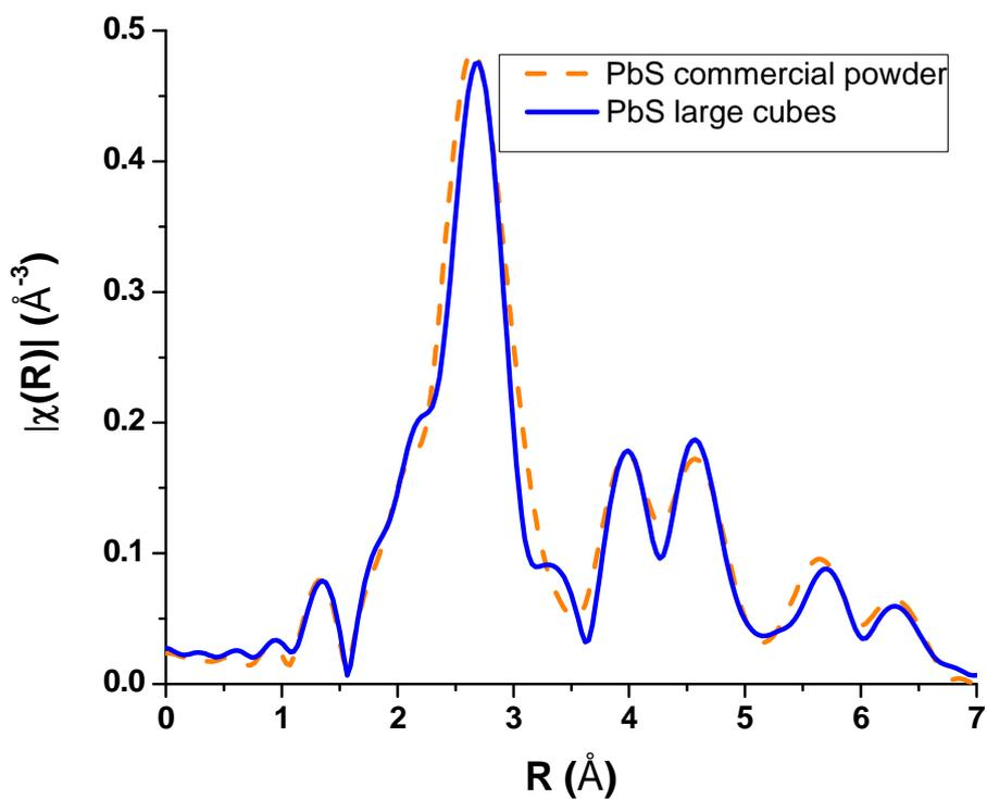
Figure 3.3:  $\chi(R)$  plot of PbS powders: the bulk commercial powder is marked in dashed orange, the large agglomerated nanocubes morphology is marked in solid blue.
