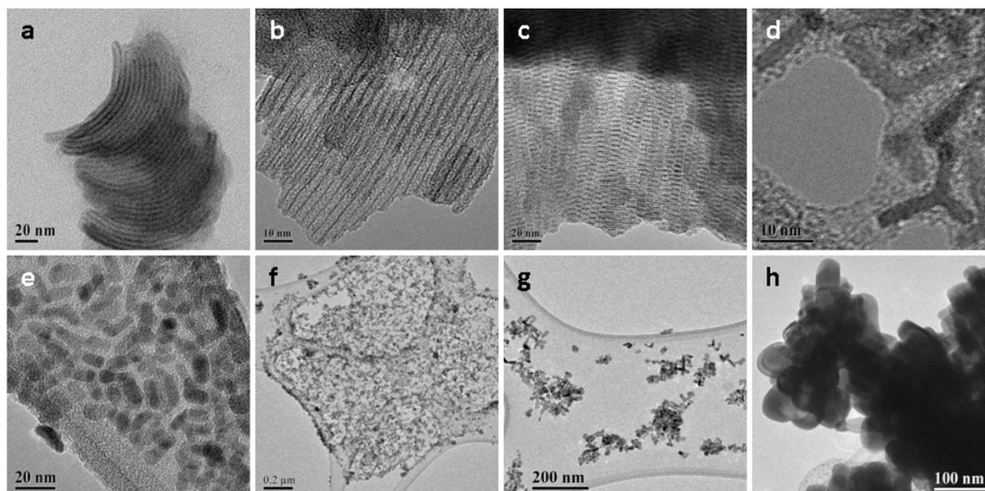
**Figure 2.1:** BF TEM images of metal sulfide nanoparticles: (a) curved ZnS wires, (b) straight ZnS wires, (c) ZnS rods, (d) CdS tripods, (e) prolate CdS rods, (f) ordered PbS cubes, (g) small PbS cubes and (h) large PbS cubes.
