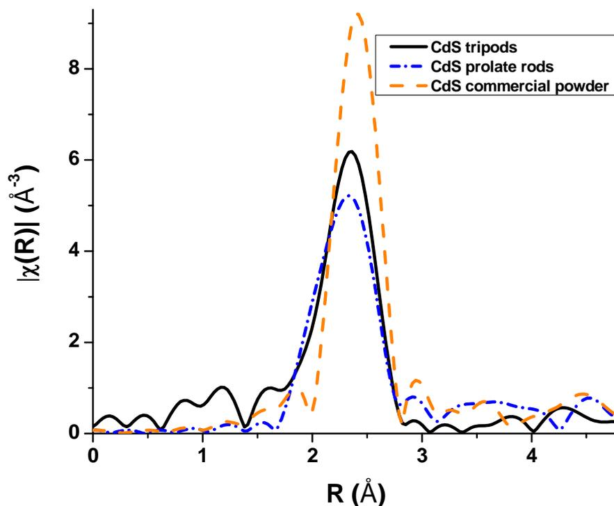
Figure 3.2:  $\chi(R)$  plot of CdS powders: the bulk commercial powder is marked in dashed orange, the prolate nanorods morphology is marked in solid black and the nanotripods morphology is marked in dot-dashed blue.
