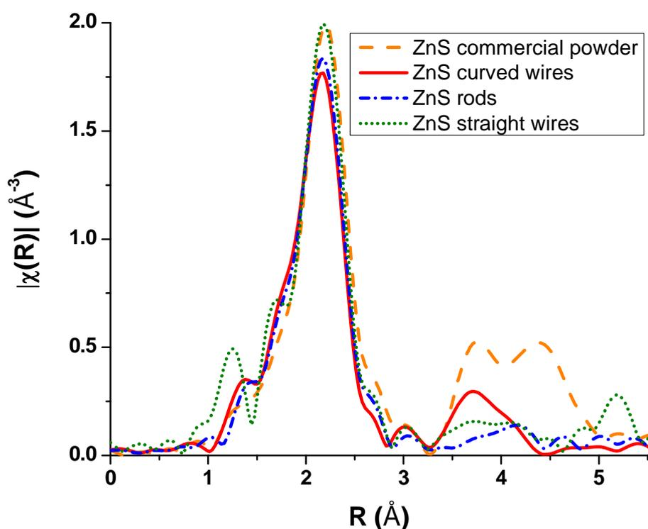
Figure 3.1:  $\chi(R)$  plot of ZnS powders: the bulk commercial powder is marked in dashed orange, the curved nanowires morphology is marked in solid red, the straight nanowires morphology is marked in dotted green and the nanorods morphology is marked in dot-dashed blue.
