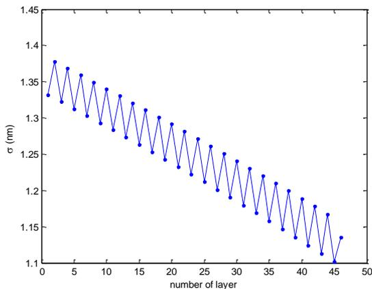
Figure 2. Dependence of interface roughness parameter  $\sigma$  on number of the deposited layer.
