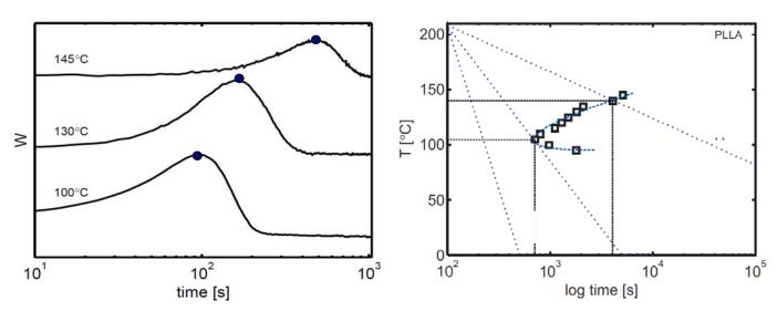
PLA are slowly crystallizing materials and with this diagram at hand, we could establish that starting from the melt at 205°C the material can be quenched amorphous at cooling rates above 8°C/min. With x-rays, we
