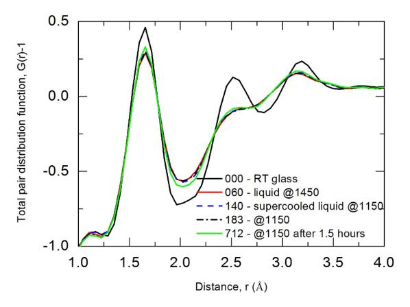
The data treatment is still ongoing. These XRD measurements as a function of time and temperature in the annealed melt before and during nucleation processes will give important parameters to understand structural rearrangement during crystallization processes and will be completed by x-ray absorption spectroscopy at the Sr K-edge at high temperature that will give information on the short range order evolution about Sr atoms.
