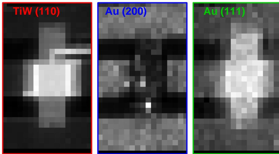
*Figure 1 : 2-dimensional maps performed on the virgin RF-MEMS at the characteristic peak of TiW(110), Au(200) and Au(111)*
