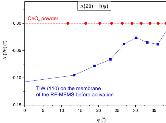
**Figure 2 : Deviation to the TiW (110) Bragg angle measured on the membrane of the RF-MEMS before activation (blue line)- and reference CeO<sub>2</sub> powder (red line) (deviation to this curve is directly attributed to residual stress in the layer)**
