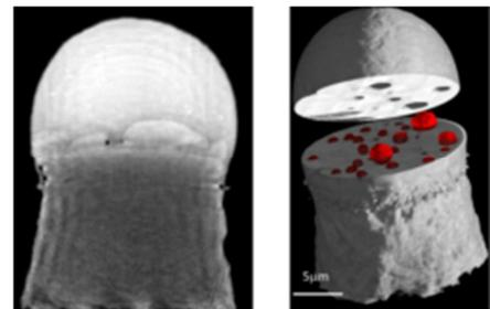
**Fig.1:** 2D sagittal slice through the 3D reconstruction (left), showing intermetallics and 3D volume rendering showing voids, in red (right)
