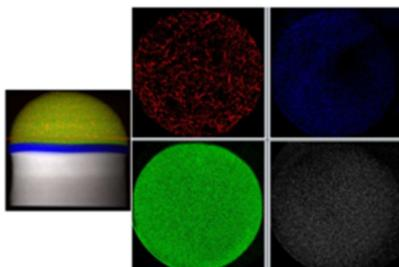
**Fig.2:** 2D fluorescence mapping of a copper pillar (left) and 4 fluorescence tomography slices. Color coding: copper, nickel, tin, silver are in gray, blue, green and red, respectively.
