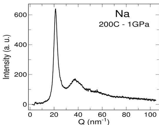
**Fig. 1** Total diffuse scattering of liquid Sodium obtained at 200C and 1GPa at ID27 using the MCC during the experiment.
