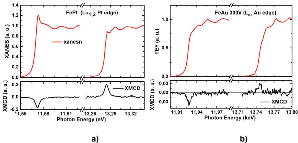
**Figure 2:** XMCD spectra obtained on annealed FePt (a) and FeAu (b) clusters at 5 d L<sub>2,3</sub> edges
