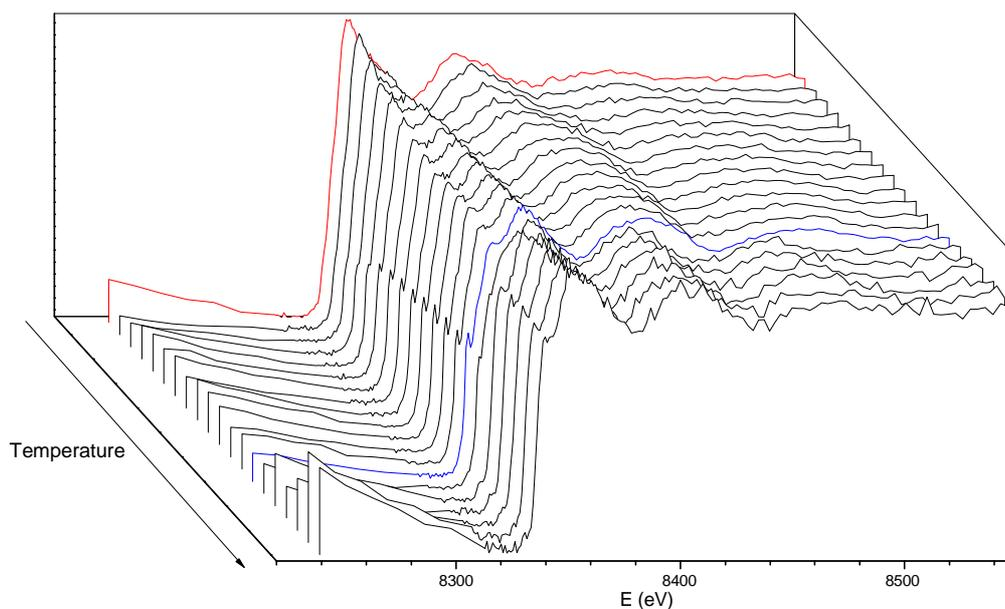
**Figure 1: in situ XANES data of the decomposition of nickel iso-butyl dithiocarbamate at a ramp rate of 1° C/min and scan time of approximately 12 minutes. Data shows a gradual change in the edge between room temperature and 170° C (between red and blue) followed by an abrupt change in edge, and post edge oscillations.**
