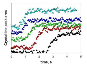
The typical sigmoidal trend of crystallinity vs. time is always observed. Remarkably, the tecnique proved to be efficient even to probe processess occurring in split seconds.
