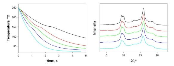
The crystallization process can be clearly identified by looking at the cooling curves (left). The temperature exhibits a deviation from the expected exponential decay with time, due to the release of crystallization latent heat. It can be noticed that, with increasing cooling rate, the structuring process shifts towards shorter times, while the crystallization temperature is only slightly affected. This is typical of polymers presenting a fast crystallization kinetics.
