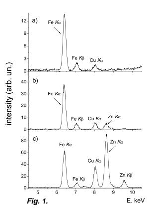
hemoglobin (Fig. 1a) and a weak peak of copper. In the spectra of thin films based on the protein treated with urea, the intensity of the peak of copper is substantially higher and, in addition, an intense peak of zinc appears (Figs. 1b, 1c). It should be noted that the intensity of the peak of Zn ions substantially increased when the protein was treated with a urea solution at a higher concentration.
