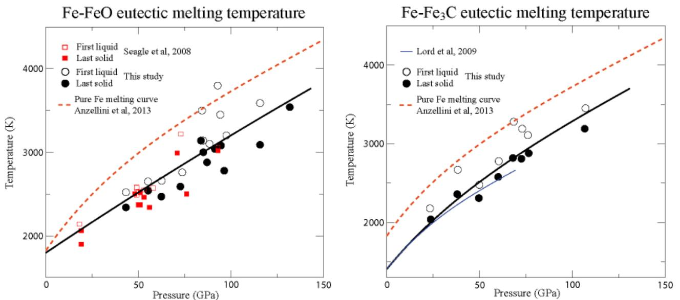
**Figure 1:** Eutectic melting temperature of Fe-O and Fe-C systems measured during HS4752 beamtime compared with previous studies (Lord et al., 2009; Seagle et al., 2008) and pure Fe melting curve (Anzellini et al., 2013).
