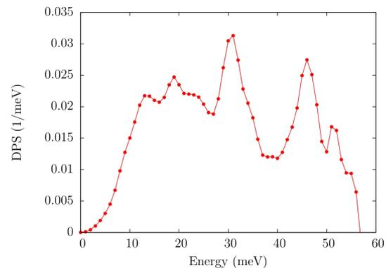
Fig.4:  $^{125}\text{Te}$  element specific DPS in  $\text{Sb}_2^{125}\text{Te}_3$  at 76.2 GPa.
