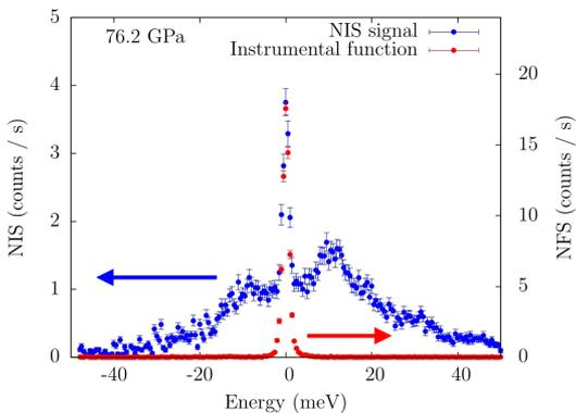
Fig.3: NIS signal and instrumental function of  $^{125}\text{Te}$  in  $\text{Sb}_2^{125}\text{Te}_3$  at 76.2 GPa.
