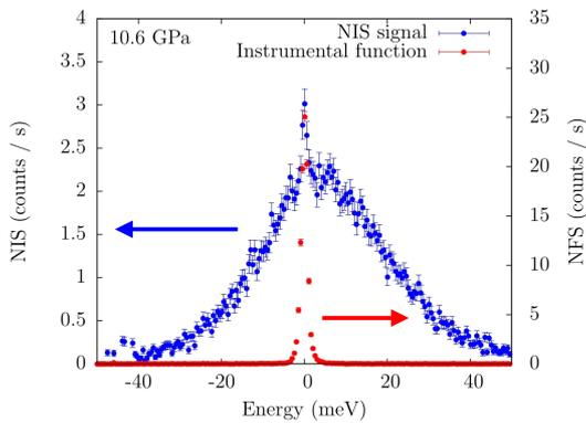
Fig.1: NIS signal and instrumental function of  $^{125}\text{Te}$  in  $\text{GeSb}_2\text{Te}_4$  at 10.6 GPa.
