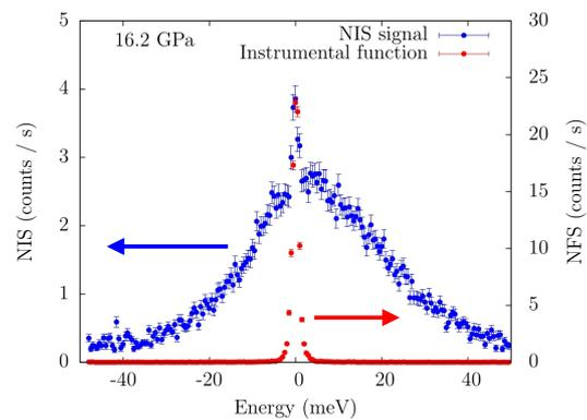
Fig.2: NIS signal and instrumental function of  $^{125}\text{Te}$  in  $\text{GeSb}_2\text{Te}_4$  at 16.2 GPa.
