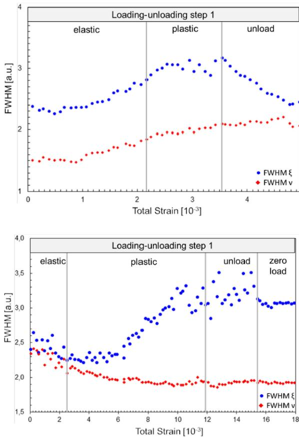
Fig. 2 Peak width evolution during the first loading step in a single crystalline sample and single crystalline with slit. In case of the single crystalline sample the peak width significantly decreases during unloading; in case of the slit it stays constant.
